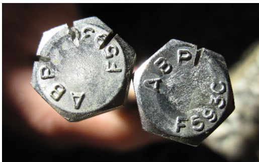
Figure 2. Examples of notched bolts used for marking permanent plots. Left bolt has 3 notches, right bolt has 1 notch. A maximum of 6 notches is recommended for hex head bolts.
