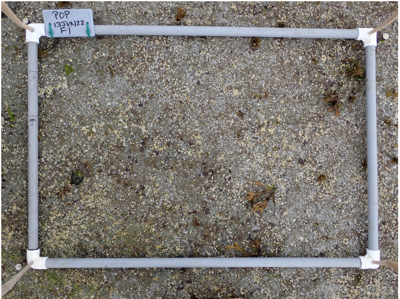
Figure 3. Example photo plot showing ideal placement of plot markers. The primary plot marker (in this case, a notched stainless-steel bolt) is in the upper left corner, and the other markers (in this case, unnotched bolts) are visible in the upper right and lower left corners of plot. This marker placement ensures consistent orientation of the photographs across repeated surveys.
